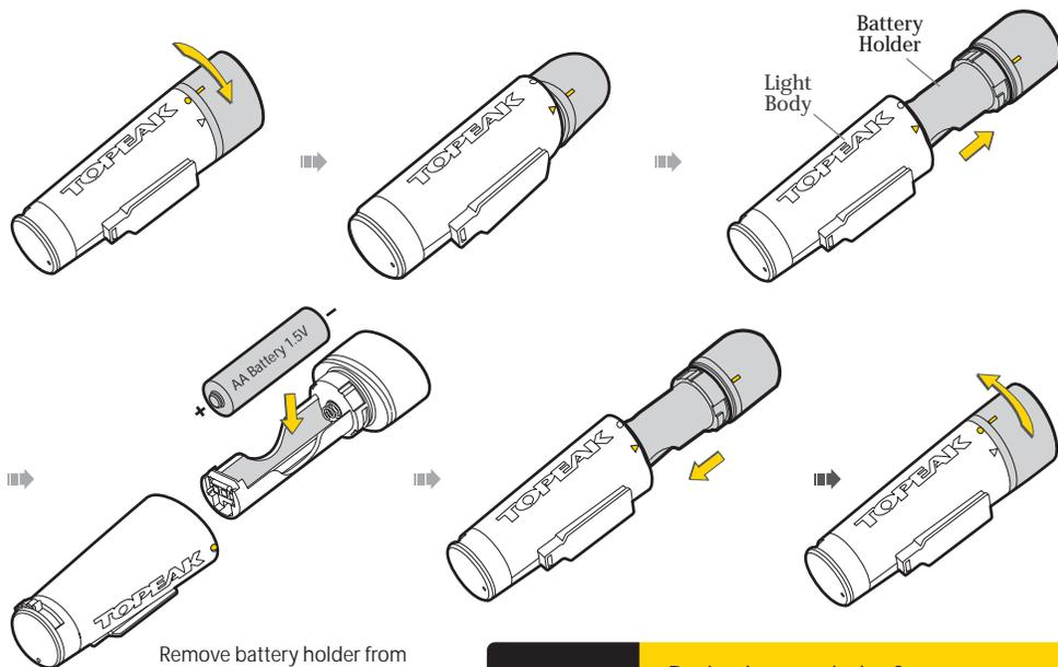
Remove battery holder from light body and insert new battery. Make sure positive and negative ends of battery is installed correctly.
